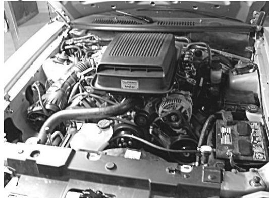
D) Once the aluminum scoop is aligned, with the hood closed, remove only the aluminum scoop from the upper air box and tighten brackets Y and Z and ball stud nut (Figure 14)
