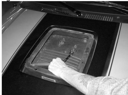
F) Assemble Shaker aluminum scoop to upper air box using two M6-1.0 x 10mm bolts. (Figure 15)
