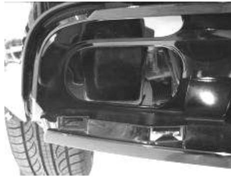
11. Install factory J-Clips, removed in step #8, onto the CDC Chin Spoiler. Note orientation of clip.
