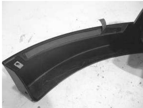
13. Align the Chin Spoiler tabs with the slots in the fascia and set the Chin Spoiler into the fascia opening. **Make sure that the pull tabs created above are accessible.**
