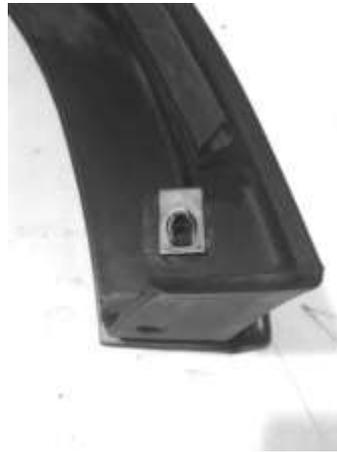
12. Create pull tabs by peeling 2"-3" of the red backing from the Acrylic Bonding Tape on the Chin Spoiler.
