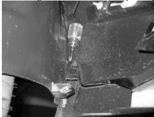
6. Remove the outside temperature sensor from the factory trim piece using a fork tool.
