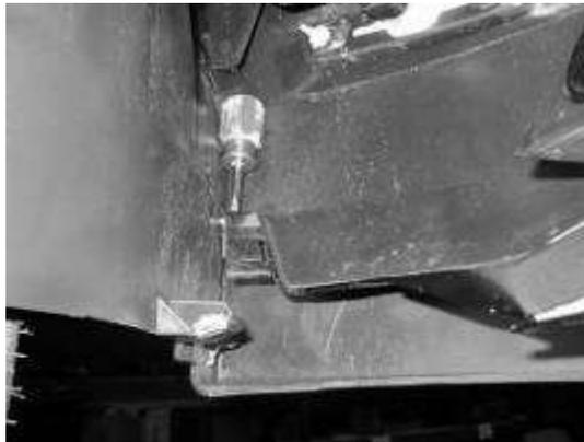
17. Secure Chin Spoiler in the wheel wells with the factory screws.
