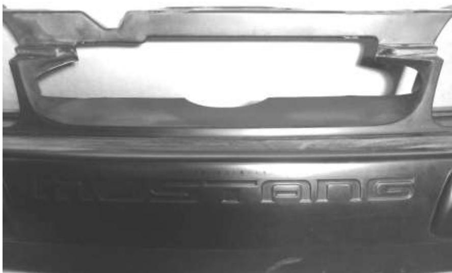
3. Remove composite structure behind the Grille opening with saw, or notch the new part to fit around the structure if you do not wish to remove.
