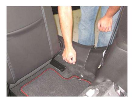
11. Remove upper and lower quarter trim panels. **A.**) Remove the upper panel the same as in Step #6. **B.**) Remove the lower panel by pulling toward the center of the vehicle to release all of the clips. **Important:** Disconnect speaker as soon as panel is released.
