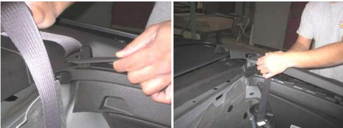
7. Drill 1-1/2" holes in upper quarter trim panels. **A.)** Cut out the provided paper template (the last sheet of these instructions). **B.)** Place panel upside down on a table and place the template as shown in picture. Mark the center point with a center punch or scribe. **C.)** Drill a pilot hole (1/8" or similar.). **D.)** Flip part right side up and drill the 1-1/2" hole with a hole saw. Do the same on the opposite side.
