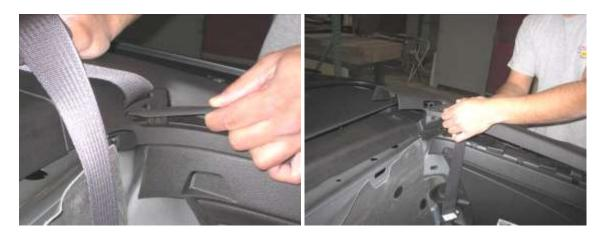
7. Drill 1-½" holes in upper quarter trim panels. **A.**) Cut out the provided paper template (the last sheet of these instructions). **B.**) Place panel upside down on a table and place the template as shown in picture. Mark the center point with a center punch or scribe. **C.**) Drill a pilot hole (1/8" or similar.). **D.**) Flip part right side up and drill the 1-½" hole with a hole saw. Do the same on the opposite side.
