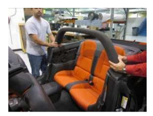
21. Tighten Set Screws. Gently press bar down on top of upper quarter trim panel and tighten set screw with a ¼" Allen wrench on both sides. **Warning:** Do not force the bar down too much as this will distort the trim panels.
