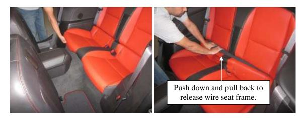
4. Remove seat back. **A.**) Refer to the picture below, use a screw driver (or similar tool) to release the metal spring clips. **B.**) Push down through the access holes and pull seat forward. Do the same for both sides. **C**) Tilt the seat down to align the slotted hinge bracket with the hinge pin of the seat. Gently pull upward to release. **Note:** There are plastic grommets in the hinge bracket that may have to be aligned to allow the hinge pin to be released.
