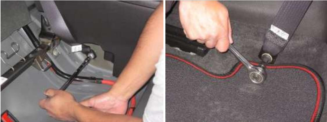
6. Remove the upper quarter trim panels. **A.)** Remove the small triangle shaped parts beneath the shoulder belt. **B.)** Gently lift straight up to release the panels and feed the seat belt through the panel.
