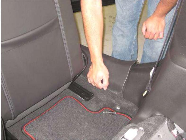
11. Remove upper and lower quarter trim panels. **A.)** Remove the upper panel the same as in Step #6. **B.)** Remove the lower panel by pulling toward the center of the vehicle to release all of the clips. **Important:** Disconnect speaker as soon as panel is released.
