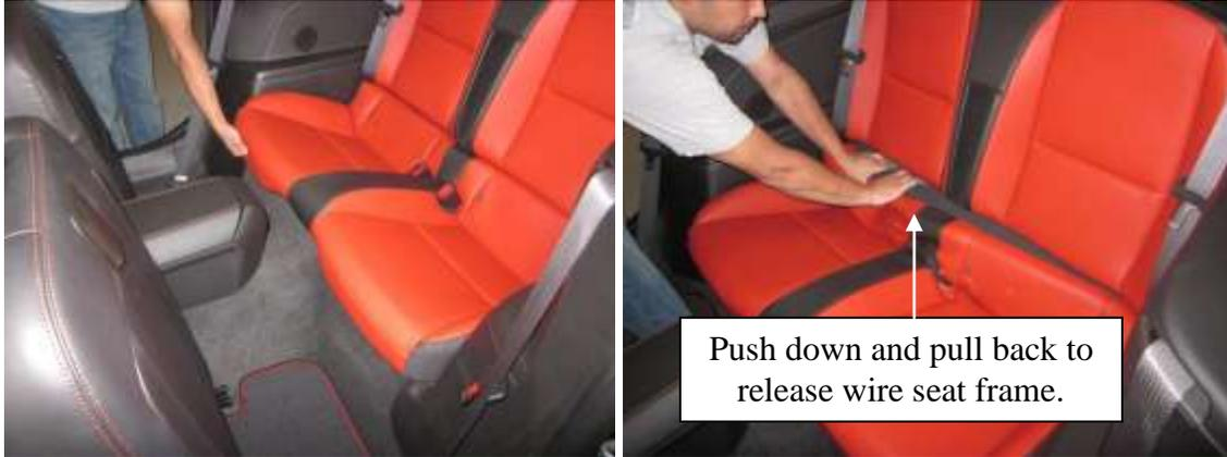
4. Remove seat back. **A.)** Refer to the picture below, use a screw driver (or similar tool) to release the metal spring clips. **B.)** Push down through the access holes and pull seat forward. Do the same for both sides. **C)** Tilt the seat down to align the slotted hinge bracket with the hinge pin of the seat. Gently pull upward to release. **Note:** There are plastic grommets in the hinge bracket that may have to be aligned to allow the hinge pin to be released.
