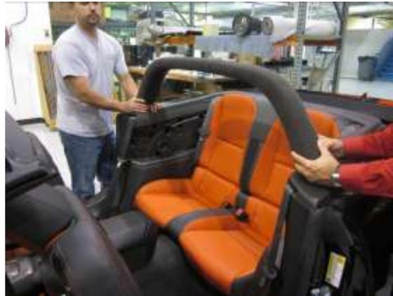
21. Tighten Set Screws. Gently press bar down on top of upper quarter trim panel and tighten set screw with a 1/4" Allen wrench on both sides. **Warning:** Do not force the bar down too much as this will distort the trim panels.
