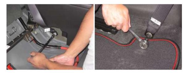
6. Remove the upper quarter trim panels. **A.**) Remove the small triangle shaped parts beneath the shoulder belt. **B.**) Gently lift straight up to release the panels and feed the seat belt through the panel.
