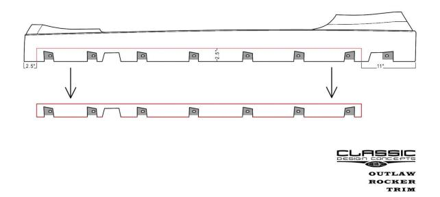
8. Remove Upper bracket from Factory Rocker. Use panel tool to separate Bracket from Rocker, this should come apart easily.
