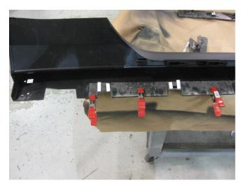
10. Using the holes in the Outlaw Rockers as drill guides, drill 3/16" holes as shown and install the supplied 3/16" rivets.
