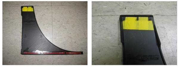
2. Assemble the Winglets to the Outlaw Rockers. <u>Note:</u> The Winglets are separate to make the painting process easier. The parts are pre-taped with 3M VHB tape. Remove the Masking tape from the back side of the Winglets, clean with the area with the supplied Alcohol Pack, and allow to dry. Apply the supplied Adhesion Promoter and allow to dry. Peel the red backing from the tape, use the alignment pins to locate the parts, and press the parts together firmly.
