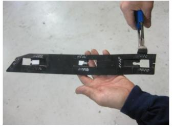
14. Clean the back side of the Outlaw Rockers, and the back side of the Bracket removed from factory rocker with the supplied Alcohol pack and allow to dry. Apply the supplied Adhesion Promoter to the same areas and allow to dry.
