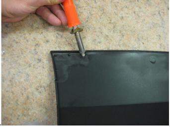
Remove the push pin retainer located at the rear of the Rocker. Remove (2) push pin retainers located at the front of the Rocker. Remove the (8) push pin retainers from the bottom of the Rocker. <u>NOTE:</u> Keep the factory retainers as they will be reused. Use a Panel Tool similar to picture below.
