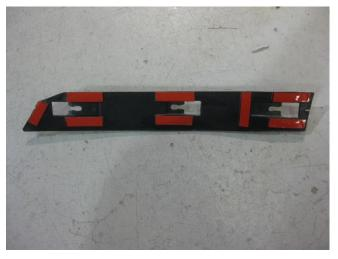
16. Remove the red backing from the 3M tape and install the bracket as shown below. **NOTICE:** There are molded alignment tabs on the Outlaw Rocker to aid the assembly. Press Bracket firmly to activate the pressure sensitive adhesive of the 3M tape.
