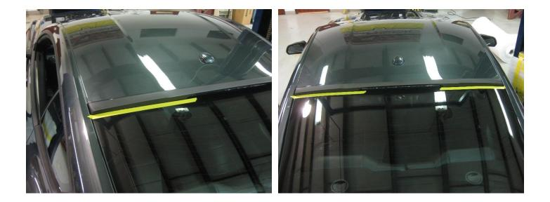
4. Remove High Mount Spoiler from car and apply the supplied **GAP-1** Adhesion Promoter. Allow time to thoroughly dry.
