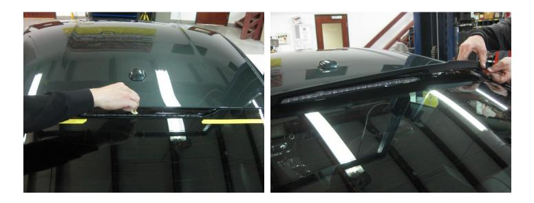
Install the High Mount Spoiler. <u>HINT:</u> The help of a friend will make this step much easier. While one person holds one side of the High Mount Spoiler down on the glass, the other person lifts their side and removes the red backing from the tape. After the backing is removed, press into position and repeat on the other side. Press firmly to activate adhesive of 3M Acrylic Foam Tape.
