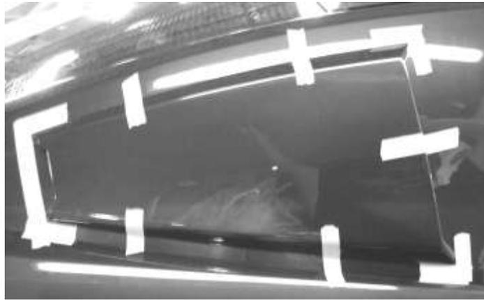
5. Remove Scoop from car and peel all red backing from the bonding tape. Install Scoop to vehicle, using masking tape as a guide.
