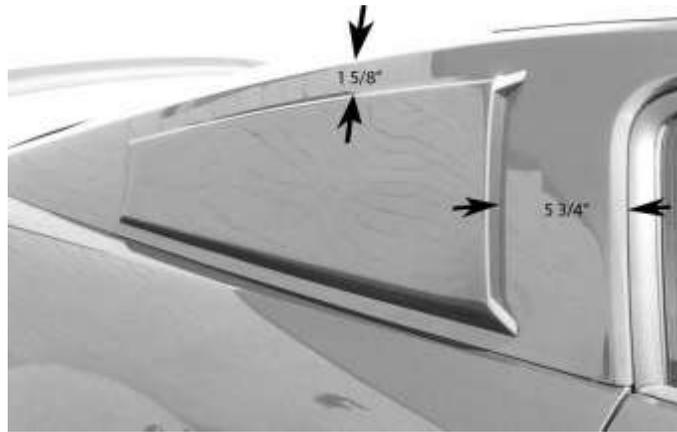
4. Once proper location has been achieved, mark the corners of the Scoop with masking tape.
