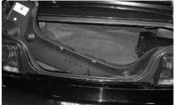
3. Remove 11mm nuts securing taillight housing to the vehicle, 3 per taillight housing. Unplug wiring harness (one connection per side). Push grommet (one per side) with wiring harness through the sheet metal from inside to outside of trunk. Remove taillight housings from vehicle.
